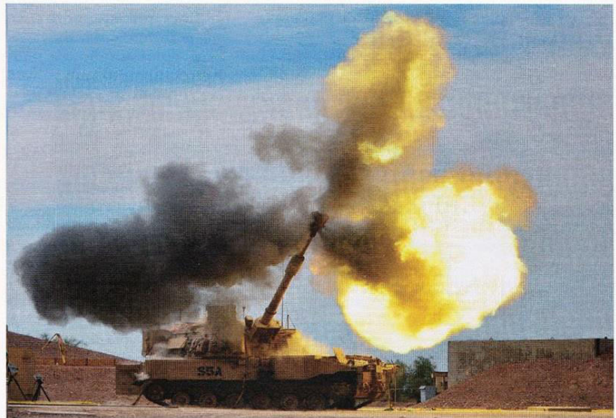
The M109A7 155 mm self-propelled howitzer fires at Yuma Proving Ground, Ariz.
