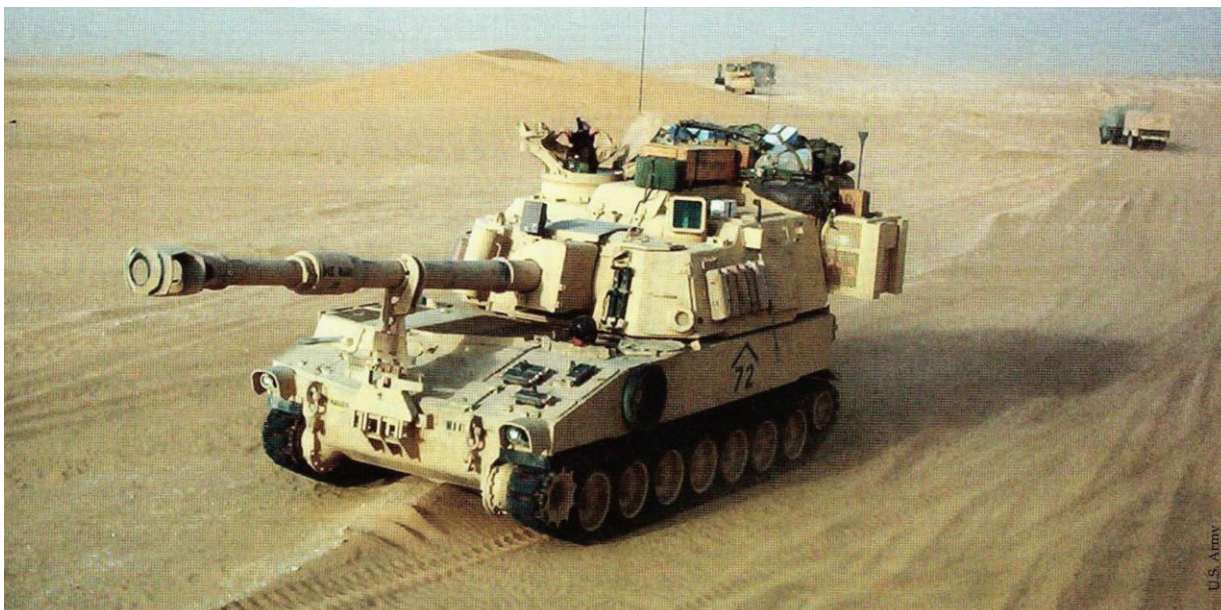
The next-generation M109 Paladin has upgraded armor and more onboard electronics.
